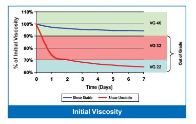
In this example, the shear unstable high VI hydraulic fluid suffered a nearly 30 percent viscosity loss in just two days and falls out of the ISO viscosity grade in less than one day of pump operation. On the other hand, a more shear stable formulation retains consistent viscosity for the duration of the test. The differentiation has a significant implication in the lubrication and operation of a hydraulics system.
